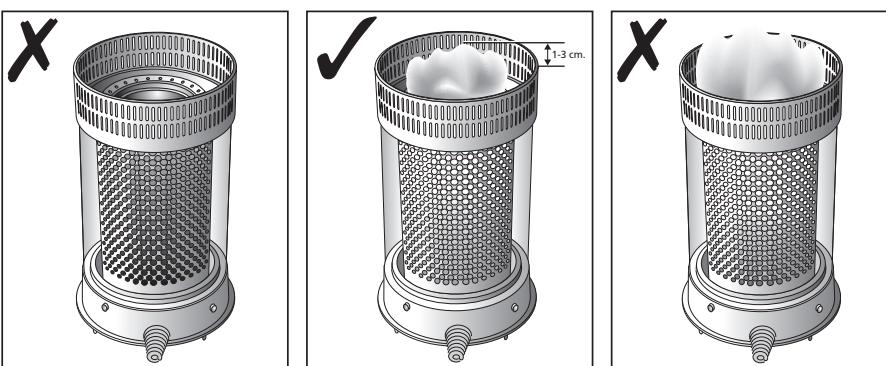
! If the flame remains low after the adjustment, the wick height must be adjusted (refer to Section G).
