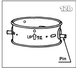
**13** Install the wick sleeve (with wick) to the primary air tube. And then turn the wick sleeve clockwise to set in the handle arm.
