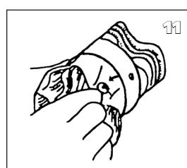
**12** Install the wick to the wick sleeve according to the allowed direction engraved on the wick sleeve.
