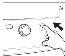
When you have ignited the heater and it shuts off again shortly after, the batteries need to be replaced. It is best to use new alkaline batteries (2x D-size).
