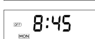
Then, use the adjustment keys 15 to set the minute. Press the adjustment key ▲ to increase the minute and the key ▼ to decrease the minute. Press extension/day/set 19 to select the right minute.
