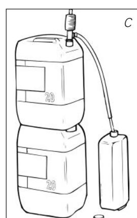
3 Fill the removable tank using a fuel pump (refer to fuel pump operation instructions.) Make sure that it is in a higher position than the removable tank (Fig. C). Insert the ribbed hose into the opening of the removable tank.
