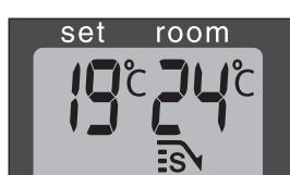
I: When the SAVE light lights up, the heater will automatically switch on or off in order to remain within a specified temperature range.
